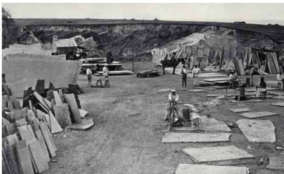
Mintaro Slate sawing yard, 1880. Hand-powered steel saws were fed with water and abrasive sand to cut the slabs to size and shape. The sloping quarry floor is at rear. (Photo 32702)
